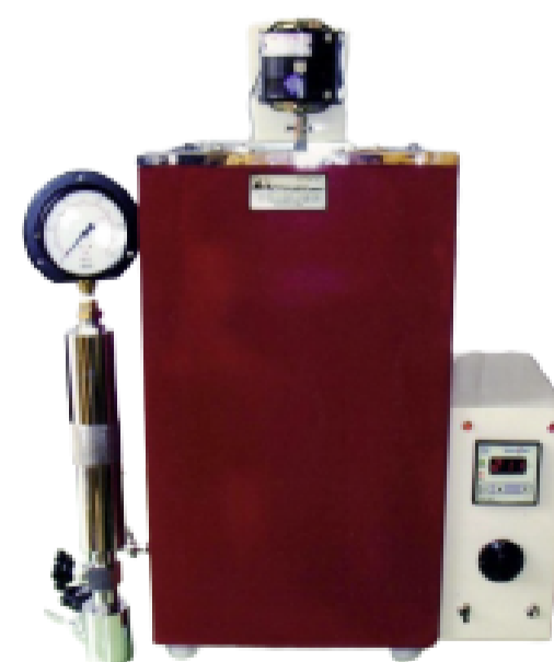
REID VAPOUR PRESSURE
